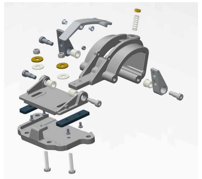
BFHHQTH-HINGE Exploded View
